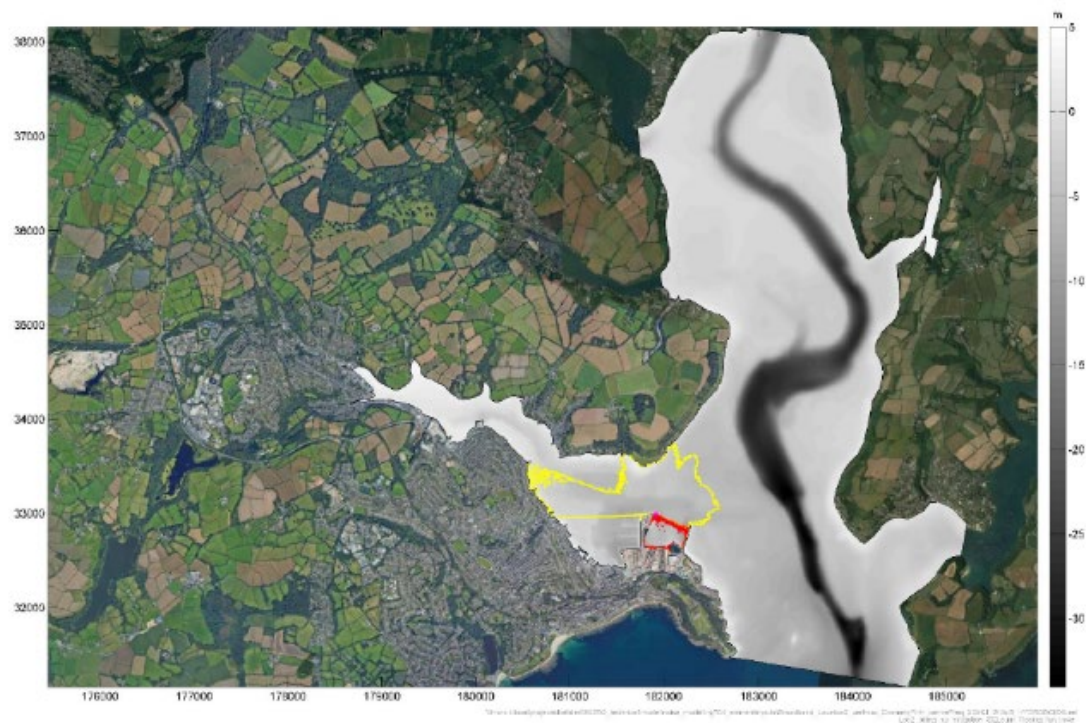
Figure 7.18: Predicted SEL cum impact footprint for fleeing fish for percussive piling, with a soft start procedure, at the Western Wharf (Location 2)
