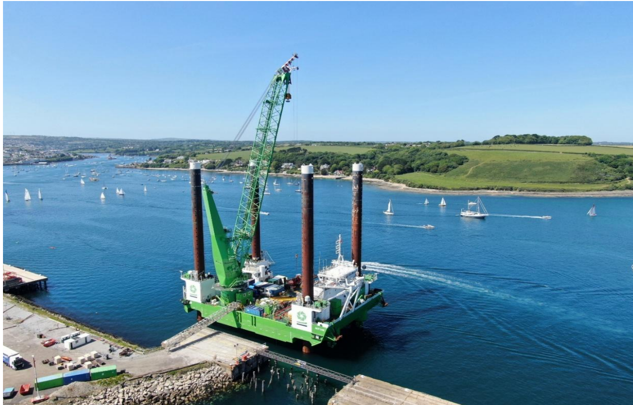
Figure 4: Neptune offshore wind GI rig adjacent to the Northern Arm
