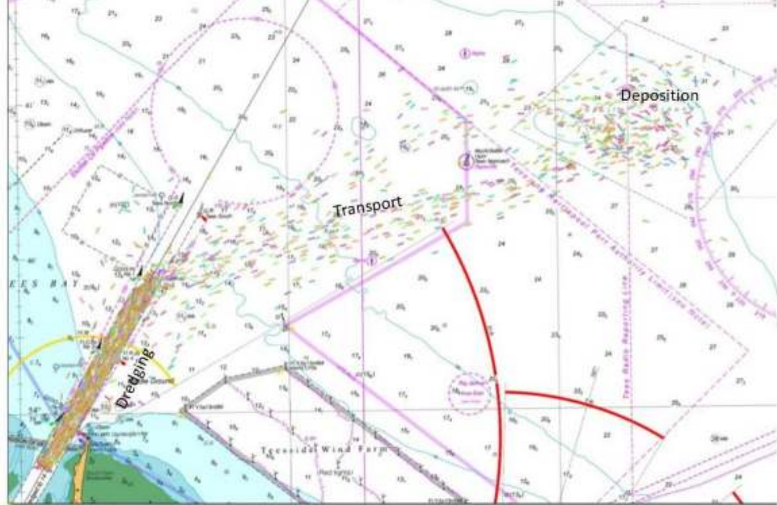
Fig 9: Compilation of the positions of the dredger over the period 25 September to 4 October every few minutes based on transmissions of its position using the AIS system. Dredging activity in the south-west and deposition site in the north-east.
