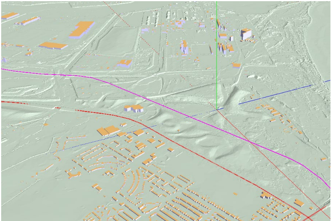
Figure E4.1: Computer model used for predicting baseline noise levels (looking north).
