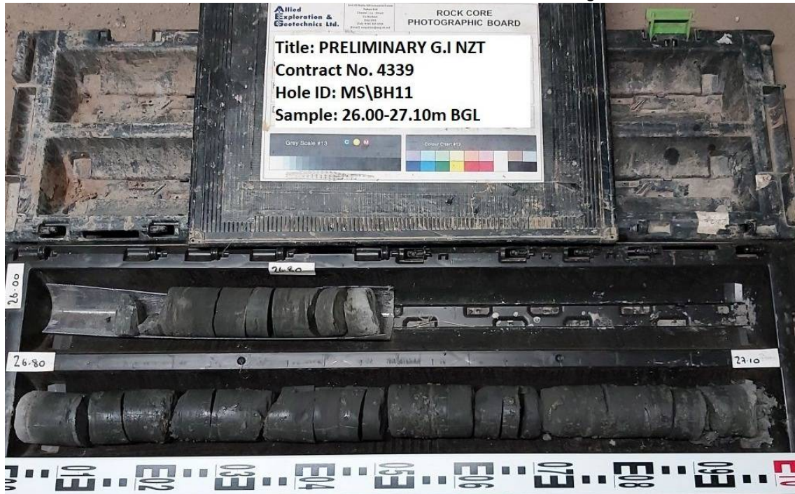
Figure MS\BH11.17 MS\BH11 26.00-27.10m BGL - Test Pocket for HDP testing
