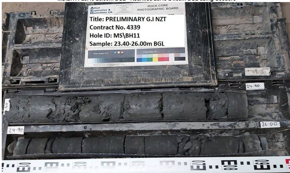
Figure MS\BH11.16 MS\BH11 23.40-26.00m BGL - Redrilled 23.40-24.50m BGL using Geobore
