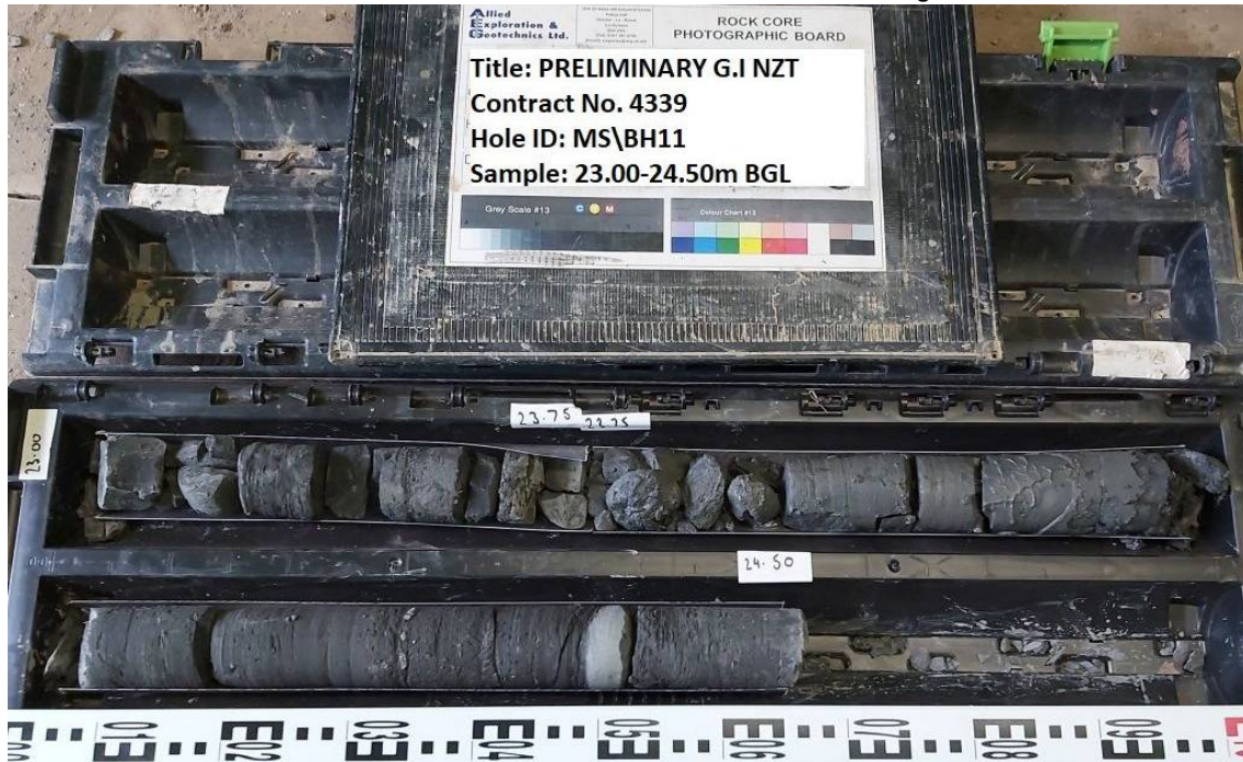
Figure MS\BH11.15 MS\BH11 23.00-24.50m BGL - Test Pocket for HDP testing
