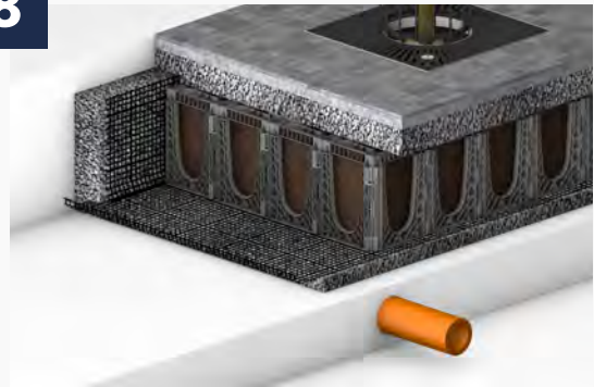
Backfill and compact to surrounding sub-base to original elevations including geotextiles.
