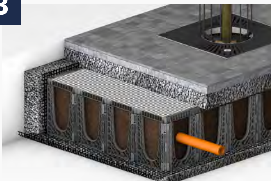
Remove aggregate subbase to expose geocomposite.
