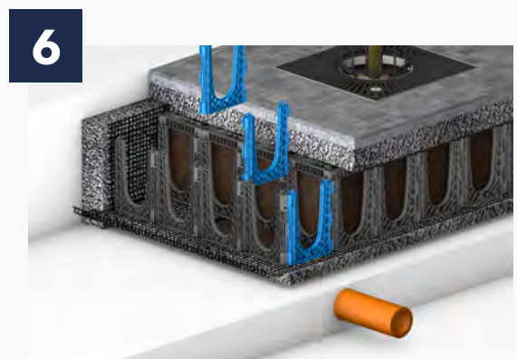
6 Remove RootSpace® Upright Panel(s) by pulling each Upright Panel up or by excavating. Remove soil.
