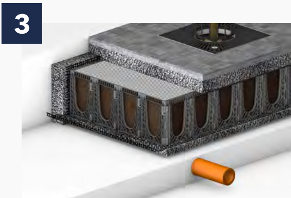
3 Remove aggregate subbase to expose geocomposite
