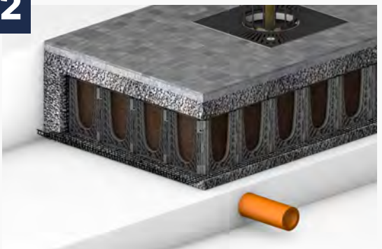
Install pavement sub-base and pavement surface.
