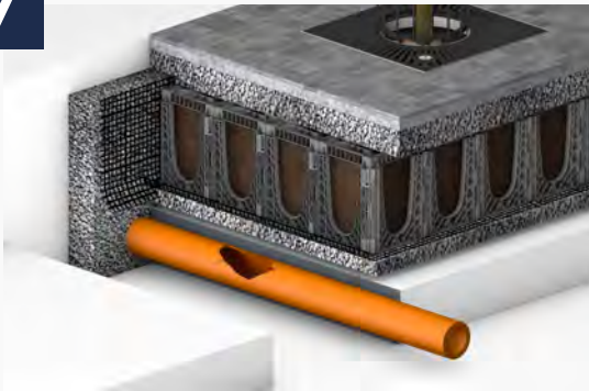
Excavate soil below RootSpace® to access and repair utility.
