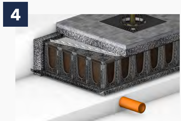
4 Cut and remove geocomposite.
