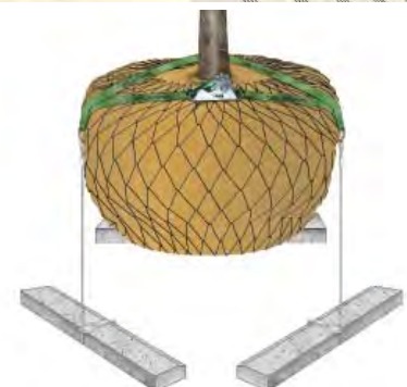
Tree Anchoring Systems: Deadman System - Plati-Mat & Strap (RF2RDMP & RF2RDMS)
