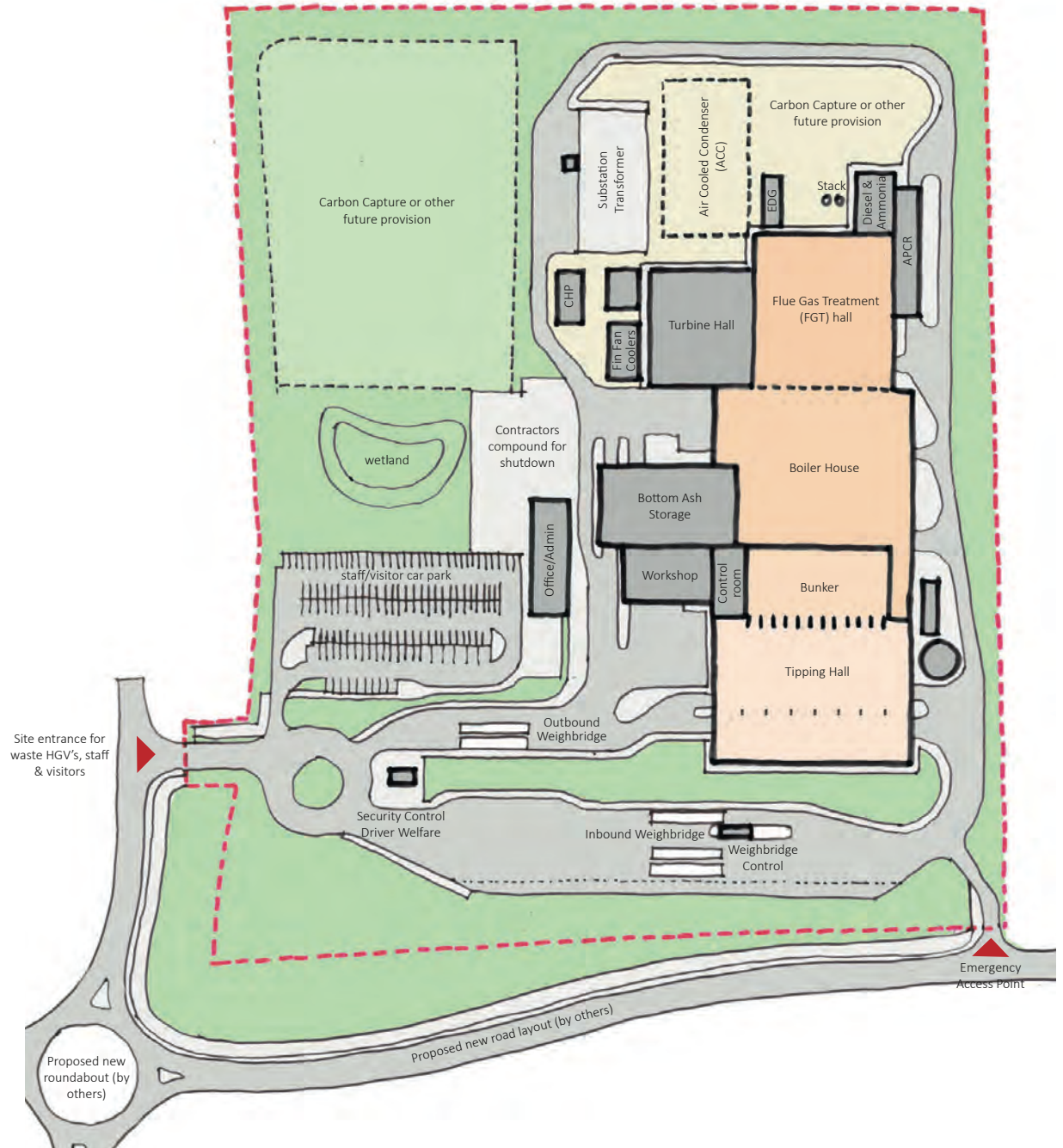
Proposed site plan diagram
